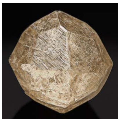
At large magnification: a spessartine crystal, also called "garnet". These are the abrasive particles that give Coticules their unique properties.
